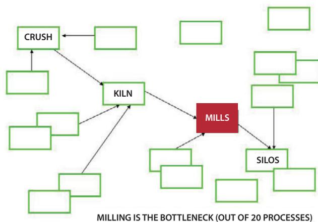
Figure 1 (left): A simplified sample diagram of critical path planning.
